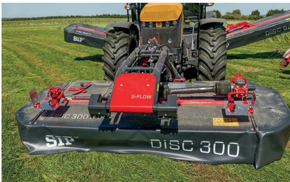
The Disc 300 front mower is pulled rather than pushed, allowing it to cope easily with uneven ground where previous mowers might have dug in. Hydraulic pressure adjustment easily achieves suitable float for any working conditions.
