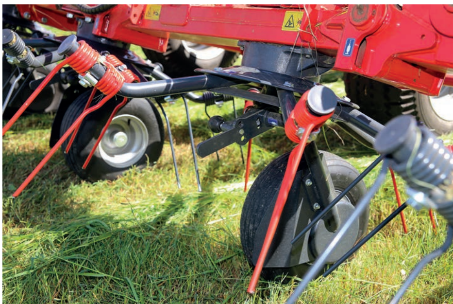
Design features such as colour coding left- and right-handed tines in black or red ensures correct selection and supply of replacements for reduced downtime. Pull out adjuster knobs have shaped profiles making them easier to grip when wet and slippery.
