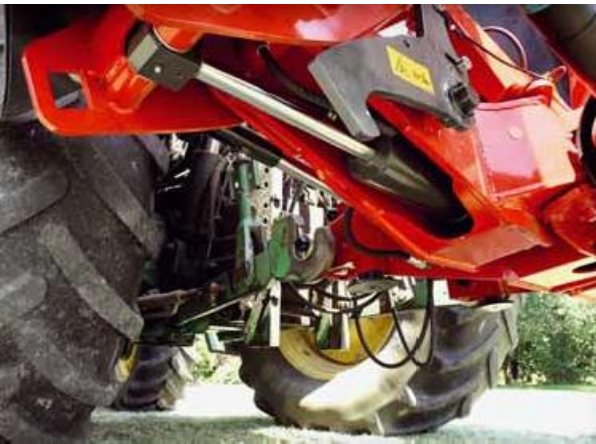
Two robust hydraulic jacks (one per unit) enable a horizontal working position with a maximum working width of 8 m (front unit included) and a 120° upward fold which can be used for road transfers (in this case the dimensions are reduced to 2.86 m ). The conditioner rollers are 2.34 m long, which makes for 81% of the working width (2.90 m).
