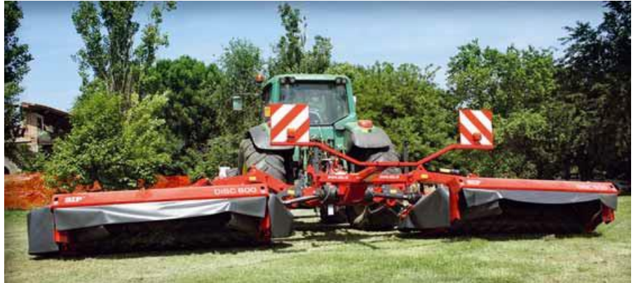
Two robust hydraulic jacks (one per unit) enable a horizontal working position with a maximum working width of 8 m (front unit included) and a 120° upward fold which can be used for road transfers (in this case the dimensions are reduced to 2.86 m ). The conditioner rollers are 2.34 m long, which makes for 81% of the working width (2.90 m).
