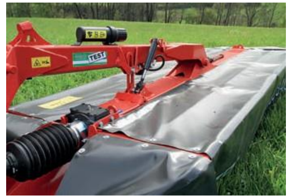
The rear mower is suspended in the middle and is hydropneumatically relieved of the load, like the front mower.
