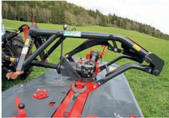
The towed S-Flow linkage of the front mower adapts to big changes in terrain even when driving fast.
