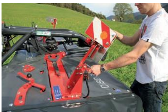
If you flip down the light racks on the front mower, you get a clear view of the mowing edge. All photos: Paar
