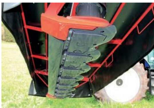
Wear skids made of Hardox steel protect the cutter bar from below.
