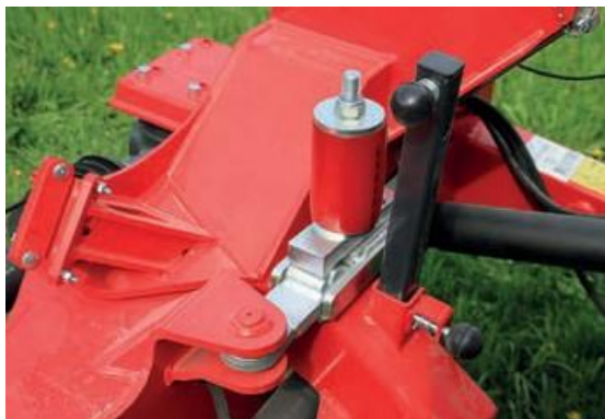
Collision protection: if you drive towards an obstacle, the bar pivots away backwards and upwards, and then returns automatically.
