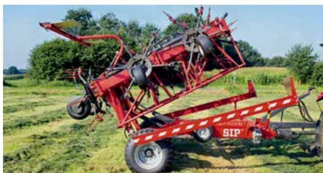
The headland spreading curtain and lights come first. Next, the 10 rotors swing over the transport axle ...
