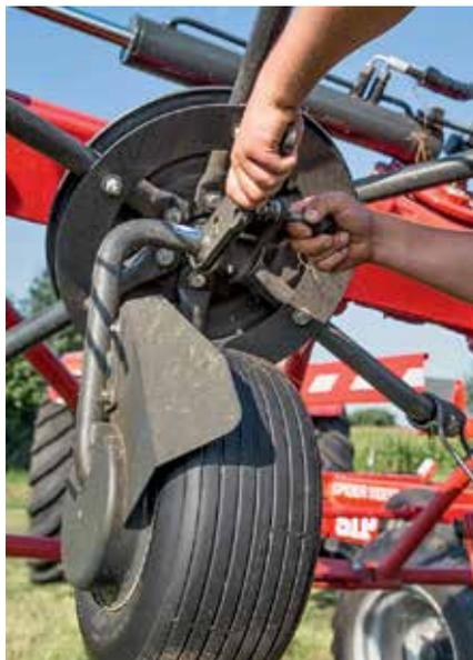
The spreading angle can be set to one of three positions.
