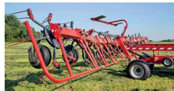
... before unfolding. The hooped frame is made from 40mm pipe with a 2.5mm wall. Everything is carried on a very strong and stable 160mm x 90mm main frame.
