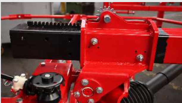
STAR 720/22: Mechanical adjustment of working width from 6,60 to 7,15m.
