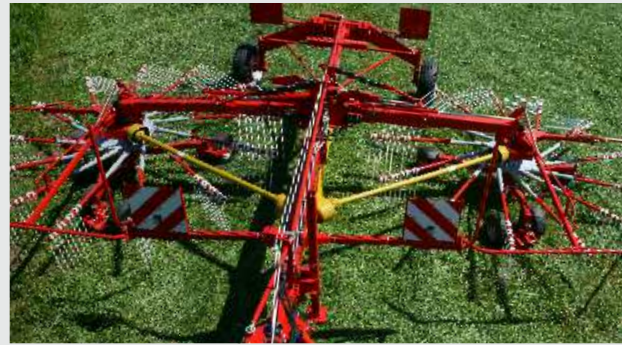
The Y-drive of the rotors enables a low working angle of the PTO shafts and a long lifespan.
