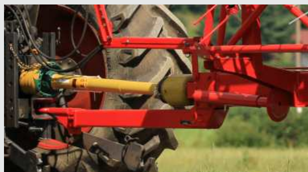
Combined drawbar for upper or lower hitch. Stable, easy-to-use parking stand.
