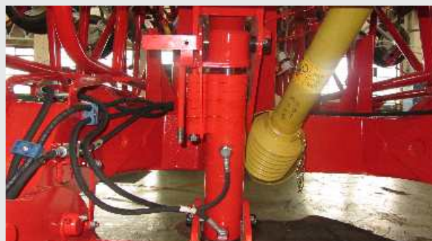
Hydraulically adjusted working height (SIP patent). Rotor angle adjustment from 10° to 19°.
