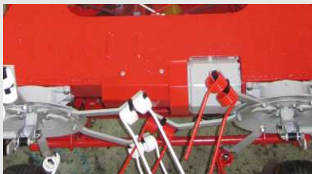
Gearbox with innovative protection system for both sides of the tedder.
