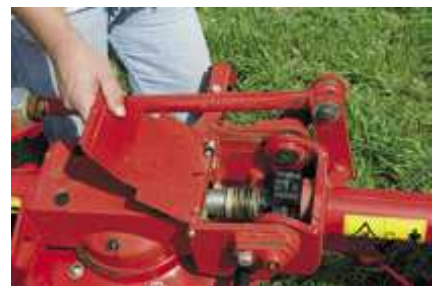
(5. photo: The force for outer rotor-segments is with finger-joints that need no maintenance.)
