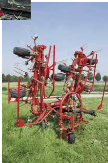
(4. photo: The stable support leg assures safe removal on less solid ground as well. Folded rotary tedder is really compact and therefore totally stable.)
