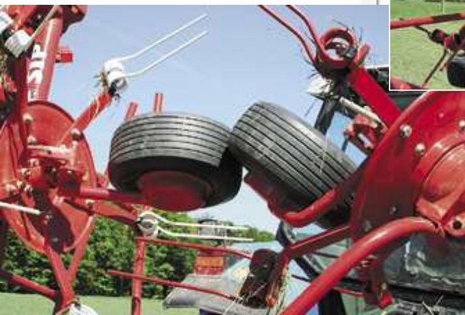
(2. & 3. photos: There could be a contact between the wheels when folding the machine. Normally they move apart after that. Contacts of the tines and wheels cause no damage.)
