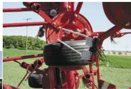
(2. & 3. photos: There could be a contact between the wheels when folding the machine. Normally they move apart after that. Contacts of the tines and wheels cause no damage.)
