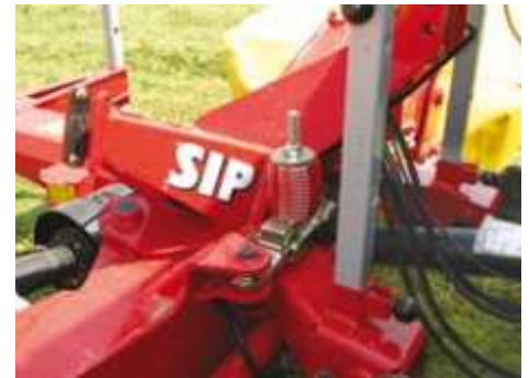
collision safety device with neoprene spring
