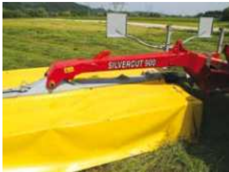
middle oscillating connection of the rear mowers' cutter bars
