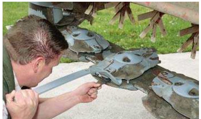
Absolutely deficient are the missing start-up protections. The curtains however can be lifted well and get arrested on their own. The intensity of the kneading machine can be adjusted five times in the hole-raster.
