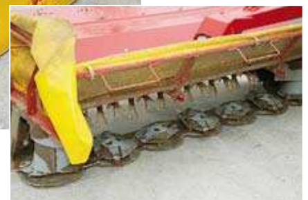
Absolutely deficient are the missing start-up protections. The curtains however can be lifted well and get arrested on their own. The intensity of the kneading machine can be adjusted five times in the hole-raster.
