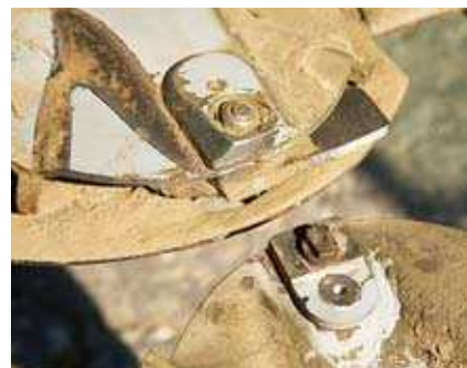
Sip bets on screwed fixing of the blades.
