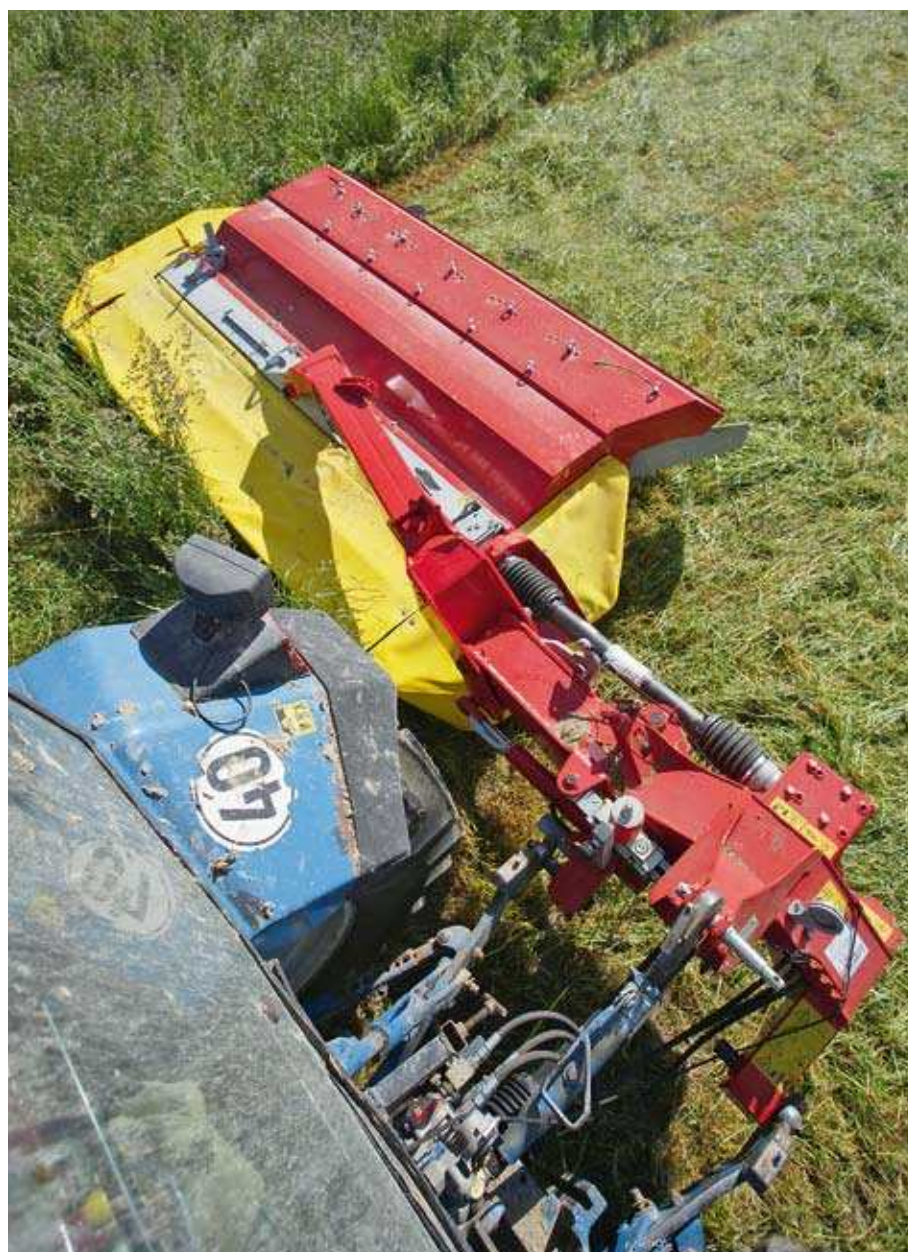
The mower from Slovenia left a good impression at our test. Also small grass was well mowed and kneaded
