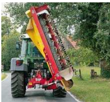
The mower is close to the tractor and extends far over on the right side. It would be better if the machine were to be folded a bit more.
