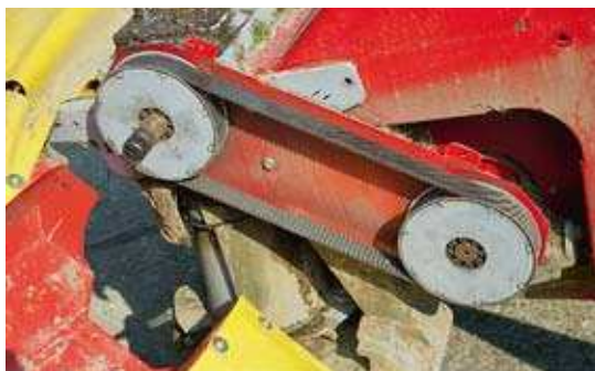
The drive of the kneading machine is performed over cogwheel belt without strain-cylinder. Straining is performed by the means of two straining-gears on the shaft of the kneading machine.
