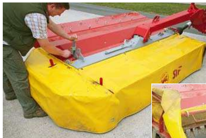
Absolutely deficient are the missing start-up protections. The curtains however can be lifted well and get arrested on their own. The intensity of the kneading machine can be adjusted five times in the hole-raster.
