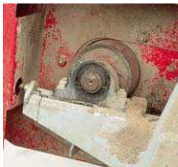
The drive of the kneading machine is performed over cogwheel belt without strain-cylinder. Straining is performed by the means of two straining-gears on the shaft of the kneading machine.
