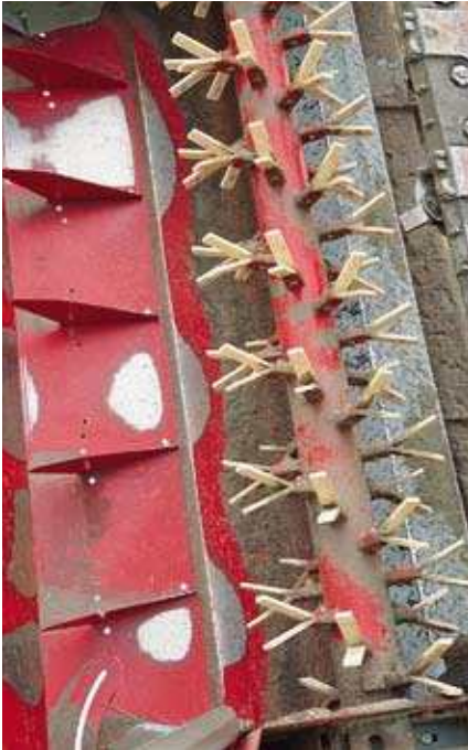
The kneading machine with Y-tines works with constant rotation. The inner guiding metal sheets can be adjusted in five levels, the outer ones with no-level in the long hole.
